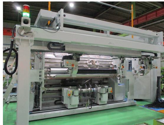
Film slitter for electronic component manufacture
