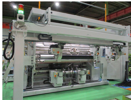
Film slitter for electronic component manufacture
